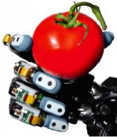
Figure 4 The Shadow Hand with tactile sensors.
