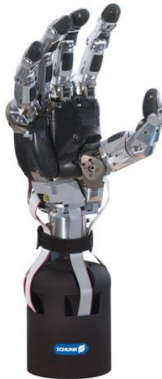
Figure 3 The Schunk Dexterous Hand.
